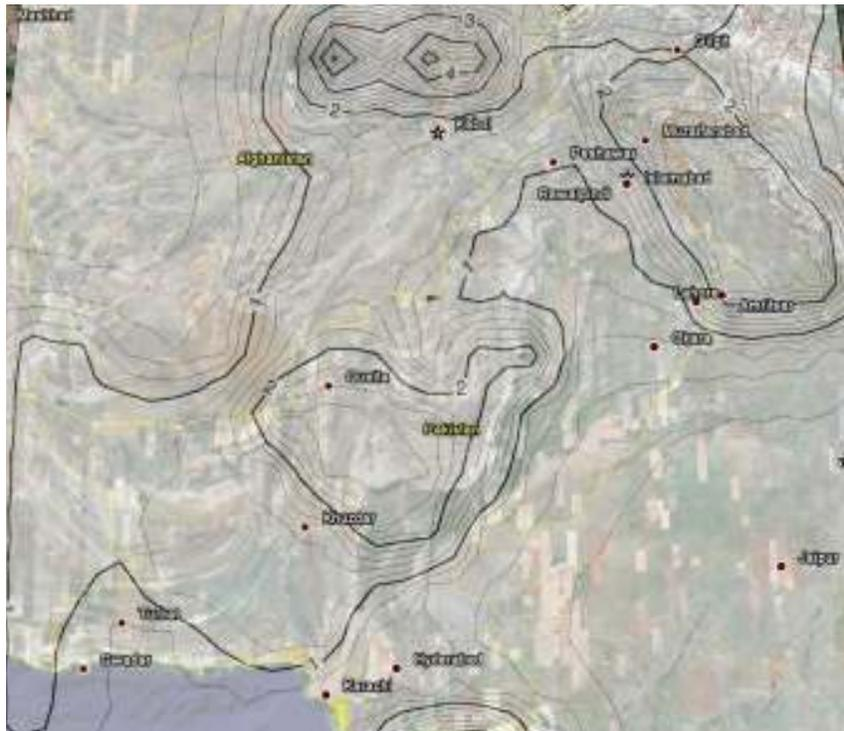
Figure 8.2. Earthquake hazard for Pakistan in terms of PGA [ $m/s^2$ ] for the 0.01 annual exceedance probabilities (100 year recurrence).
